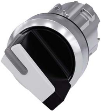
Selector switch, illuminable, 22 mm, round, metal, shiny, white, selector switch, short, 2 switch positions O-I, latching, actuating angle 90°, 10:30h/13:30h
