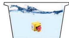
IP67: Submersion to one meter for 30 minutes.
