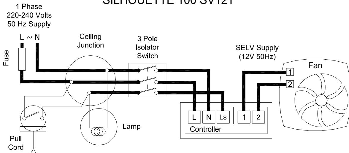
IMPORTANT "Ls" SIGNAL MUST BE THE SAME PHASE AS THE MAINS INPUT PHASE.
