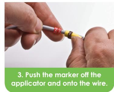
3. Push the marker off the applicator and onto the wire.
