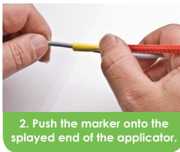
2. Push the marker onto the splayed end of the applicator.
