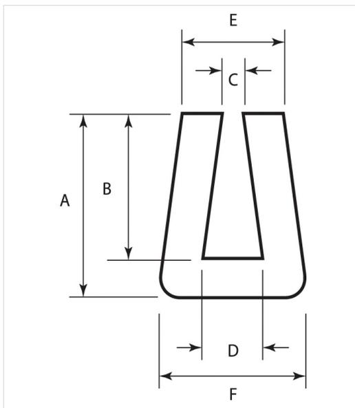
Made from self-extinguishing PVC, this material has excellent flexibility which makes application quick and easy. A halogen-free type is now also available for use in critical areas.
