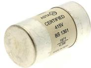
**Fuse-link, low voltage, 60 A, AC 415 V, 33 kA, BS system C type II, 30 x 57 mm, gL/gG, BS**
