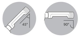
It is recommended to employ a slight "rocking" motion whilst drilling. This helps with cooling and dust removal.
