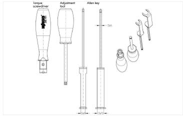
Assembly kit for pre-assembled IP67 cables and hex nut connectors (756 Series) consists of:
