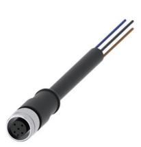
Connecting cable with M12 socket 5-pole and free cable end, 5 m long for connecting position switch 3SE51/52 wired with M12 connector 5-pole
