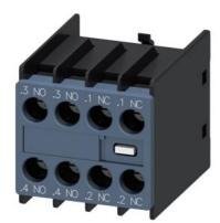
auxiliary switch, on the front, 2 NO + 2 NC, .3/.4, .3/.4, .1/.2, .1/.2, current path: 1 NO, 1 NO, 1 NC, 1 NC, screw terminal, for contactors 3RT2 and contactor relays 3RH2
