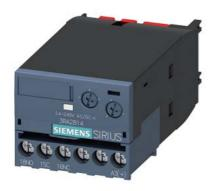
solid-state time-delayed auxiliary switch, off delayed, with control signal, relay: 1 CO, time range 0.05-100 s, 24-240 V AC/DC, 50/60 Hz, varistor for attenuation of the contactor coils integrated, screw terminal, can be snapped on at the front on contactors 3RT2 and auxiliary contactors 3RH2
