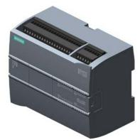
SIMATIC S7-1200, CPU 1215C, compact CPU, DC/DC/relay, 2 PROFINET ports, onboard I/O: 14 DI 24 V DC; 10 DO relay 2 A, 2 AI 0-10 V DC, 2 AO 0-20 mA DC, power supply: DC 20.4-28.8 V DC, program/data memory 200 KB
