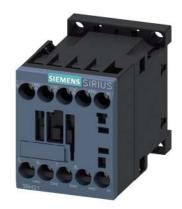
Contactor relay, 2 NO + 2 NC, 110 V AC, 50 Hz, 120 V, 60 Hz, Size S00, screw terminal
