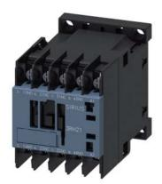
Contactor relay, 2 NO + 2 NC, 200 V AC, 50 Hz, 200 .. 220 V, 60 Hz, Size S00, ring cable lug connection
