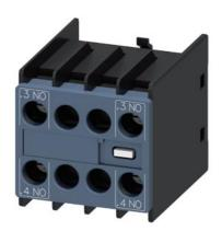
auxiliary switch, solid-state compatible, on the front, 2 NO, .3/.4, --/--, .3/.4, current path: 1 NO (solid-state compatible), --, --, 1 NO (solid-state compatible), screw terminal, for contactors 3RT2 and contactor relays 3RH2
