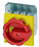
SENTRON, Switch disconnector 3LD, emergency switching-off switch, 4- pole, lu: 32 A, operating power / at AC-23 A 400 V: 11.5 kW, front-mounted, rotary operating mechanism, Red / yellow, 4-hole mounting of the handle
