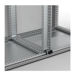
**Omschrijving:** Fitted in the centre of a 1200 mm or 1600 mm wide enclosure (top and bottom), to provide standard mounting facilities in two sections of 600 mm or 800 mm wide. This enables separate fitting of accessories such as CAB(P), CBU, CLPK, CLPF etc., in either side of the enclosure. Accessories are adjustable in depth within the 25 mm hole pattern.
