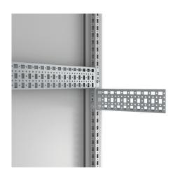
**Omschrijving:** Universal profile for both depth and width fitting on the 25 mm DIN hole pattern of the enclosure's frame or in combination with the CLPF and VB profiles. The 75 mm wide profile is equipped with three rows of holes of which one is turned 90°. This makes it possible to mount the CLPF profiles in both directions. The CLPK can be secured by the use of self tapping screws.
