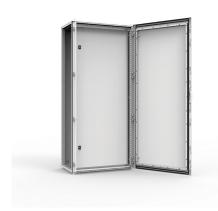
**Omschrijving:** Inner door provides a hinged mounting surface for equipment behind a standard or glazed front door. A mounting space of 80 mm, is available between the doors when the inner door is in the forward position. Can be adjusted in depth by steps of 25 mm. The mounting plate remains usable behind the inner door. The door is equipped with two double-bit 3 mm locks, and plastic handles.
