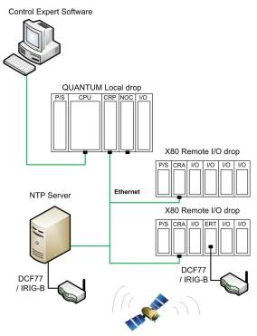
In this example, the Quantum Ethernet I/O architecture contains 2 Modicon X80 (Modicon M340) Ethernet I/O drops.
