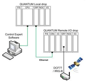
In this example, the Quantum Ethernet I/O architecture contains a Quantum Ethernet remote I/O drop.
