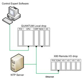
In this example, the Quantum Ethernet I/O architecture contains a Modicon X80 (Modicon M340) Ethernet I/O drop.
