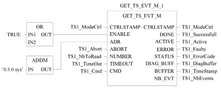
In this example the function block addresses a BMX ERT 1604 T module in the local drop. The ADDM IN parameter value ('0.3.0.sys') means the following:
