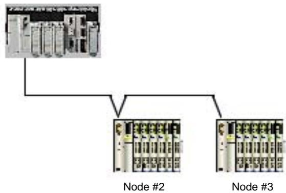
Node #2 consists of a STBNCO2212 CANopen interface module, a STBPDT310 power supply module, a STBDDI3410 4 bit input module, and a STBDDO3410 4 bit output module.
