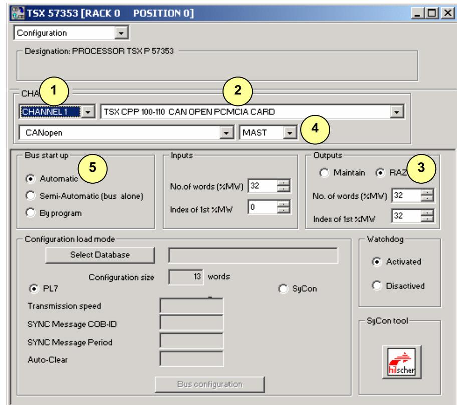
Start PL7, configure the hardware and double click on the PCMCIA slot of the CPU
