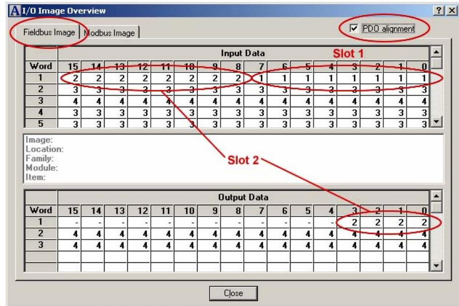
Do the same for Node #2. Make a hardcopy of both screens as it helps in understanding the IO mapping.
