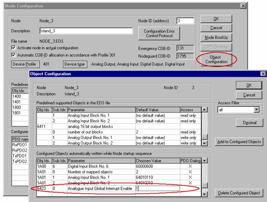
Close the window and save the project. You have now finished the CANopen configuration with SyCon and created the necessary data required by PL7 to configure the TSX CPP110 module.
