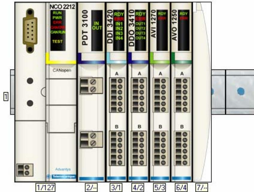
Note: You can read out the configuration when you are in online mode. In this case, the power supply module and the termination plate will be missing as they cannot be detected on the island's backplane. You must add them manually.
