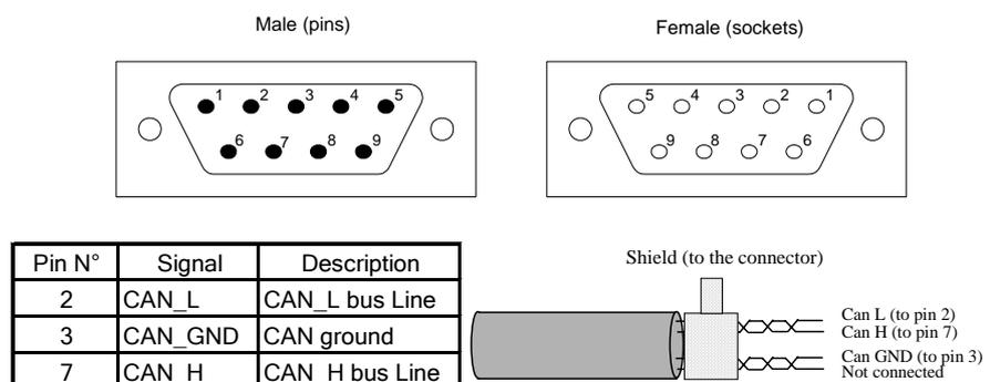
Pins 2, 3, and 7 must be connected.
