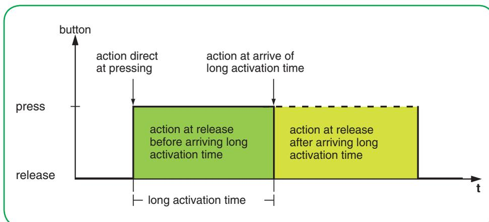
You set the relevant action for each operation phase. In addition to the normal edge function, you can set a cycle time for each object. You can send once or cyclically. You can use the action *Sends value 1 and then value 2 after a cycle time* to send a second value after a delay.
