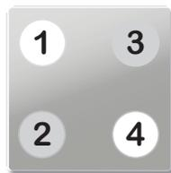
The LEDs can also be switched off. If the proximity function is activated and no proximity is detected, all LEDs are switched off. In night mode, the default setting is for only 1 LED to be switched on.
