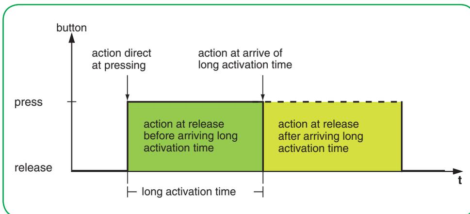
You set the relevant action for each operation phase. You can set 2 values for the scene address for each scene object. For both values, you can set whether the scene is called up or saved. The appropriate value for saving a scene is automatically derived from the scene address.
