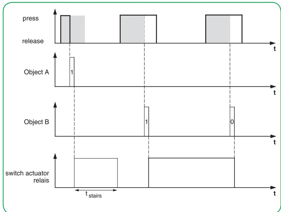
Application example for setting the staircase lighting time
