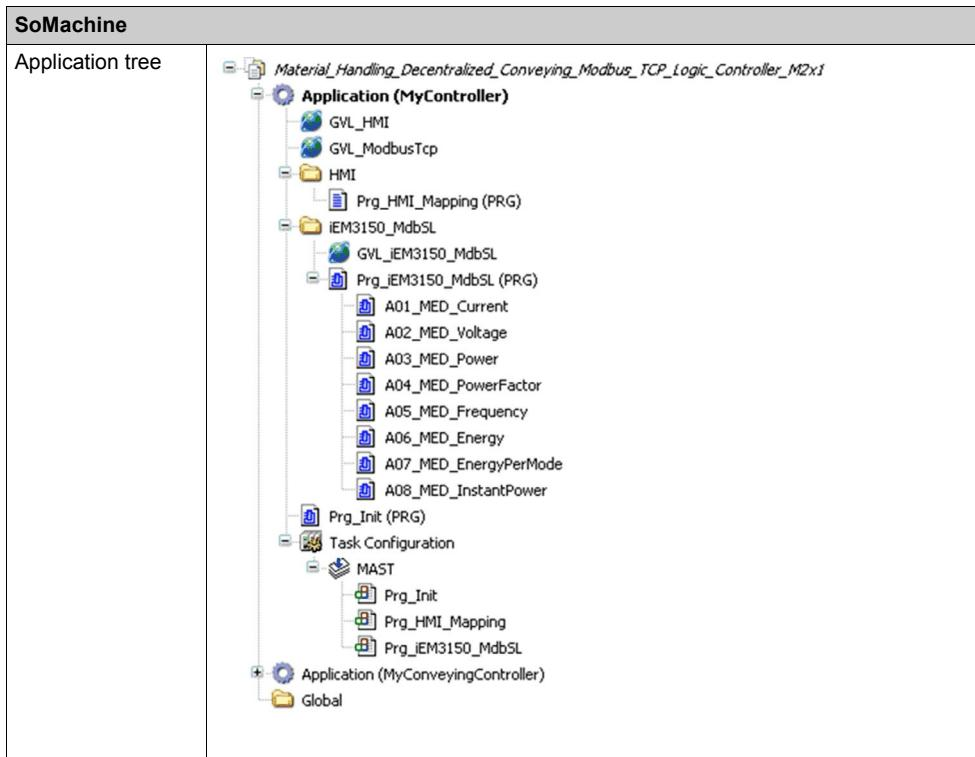
The SoMachine application tree for the Modicon M251 Logic Controller consists of two main applications parts:
