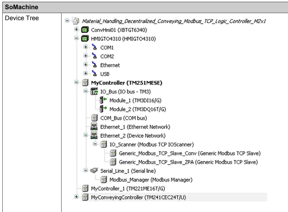
The embedded IO\_Scanner (Modbus TCP IOScanner) is linked to the port Ethernet\_2 (Device Network). Therefore, this Ethernet port is used to READ/WRITE data to and from the Modicon M241 Logic Controller and Modicon M221 Logic Controller.
