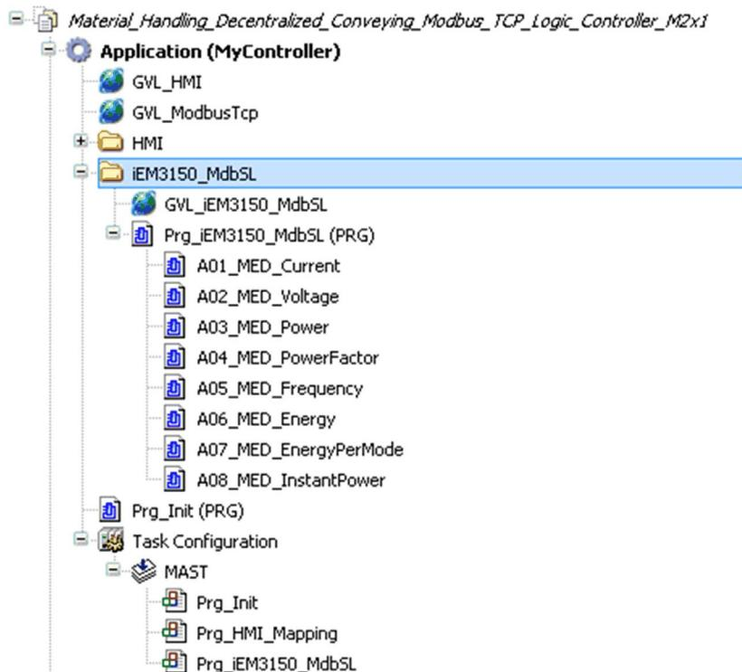
The program POU Prg\_iEM3150\_MdbSL reads energy values provided by the iEM3150 power meter and links them to the relevant application function blocks (AFBs) provided with Machine Energy Dashboard library.
