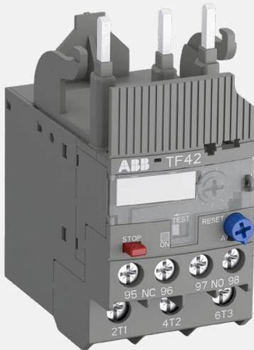
ABB's TF42 thermal overload relays are economic electromechanical protection devices for the main circuit. They are used mainly to protect motors against overload and phase failures. Starter combinations are setup together with contactors.
