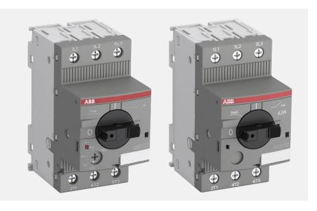
ABB's MS132 manual motor starters and MO132 manual motor starters magnetic only are electromechanical protection devices for the main circuit. They are mainly used to provide fuseless protection of motors against short-circuits, overloads and phase failures. In addition, they are used to switch motors ON/OFF manually. Starter combinations are setup together with contactors and are available with screw or Push-in Spring terminals.
