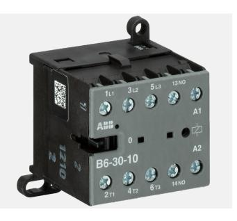
ABB's B6/BC6 mini contactors are reliable switching devices characterised by very small dimensions. Mainly dedicated to the control of motor and resistive loads. The range includes standard and reversing contactors equipped with 3 or 4 main poles. B6/BC6 mini contactors are in different types of terminals available and have a wide range of accessories.
