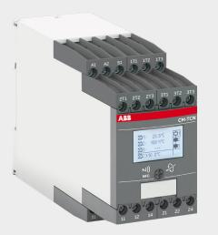
The temperature monitoring relays CM-TCN are equipped with up to three sensor circuits that accommodate inputs from the most common sensors (PTC, PT100, PT1000 and NTC). The CM-TCN relays are used to monitor the temperature of electric motors, control cabinets, busbars and to protect transformers from overheating.
