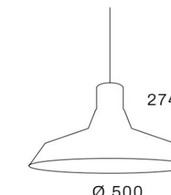
Industrial crafted LED pendant in vintage black outside and matt white inside. Suspension length 2m. Supplied with ceiling cup, also available in a 3-circuit track version. Equipped with Philips Fortimo LED module and Philips Xitanium LED driver.
