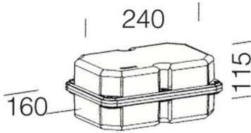
watertight box in nylon. Containing electromechanical transformer and terminal block.
