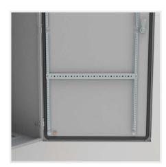
$\textbf{Description:} \ \ \text{Horizontal profiles with 25 mm hole pattern of 4.5 mm and 6.5} \\ \ \ \text{mm of diameter for the attachment and installation of equipment.}$
