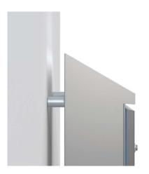
**Description:** Mounting brackets for hygienic wall fixing. Provides an space between the enclosure and the wall to facilitate cleaning operations. It includes the sealing washers to guarantee the IP rating. Machining required. Design according to EHEDG standards.
