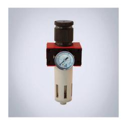
**Description:** Air pressure regulator with pressure dial, and manometer to adjust the air pressure. It filters condesated water and particles (>5 $\mu$ ). Maximum inlet pressure 13 bar, and at max pressure maximum temperature: 40 °C. Connection 1/4".
