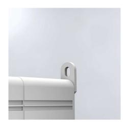
$\textbf{Description:} \ \ \text{Mounting brackets for wall fixing. Can be mounted in three different directions and will support approximately a load of 600 N.}$
