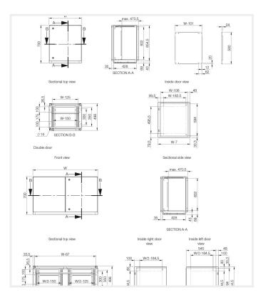
This stainless steel combinable console system, MPCS, has a IP 55/56 protection degree. It includes three interchangeable sections, top, desk and bottom. The system is very flexible and the various possible combinations can meet many design requirements. The ergonomic design of the top and desk units allows for easy installation and access to HMI-equipment, plus increases the mounting space available. This console can be installed in virtually any environment, grade dependent.
