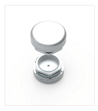
The pressure compensation plug equalises the pressure that occurs, due to temperature differences, inside the enclosure with the outside environment, while reducing the risk of dust entering the enclosure.
