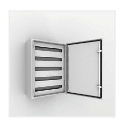
**Description:** Used for easy mounting of DIN-rail components with a maximum height of 68 mm. Distance between rows 125 mm. If required, the standard enclosure door can be replaced with a glazed door. Usable depth between front cover and external door: 35 mm. In stainless steel enclosure machining is required.
