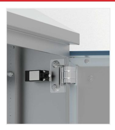
Door switch to activate any electrical device (lighting, signalling, alarms, etc.) designed for HDW wall mounted enclosures. Cable entry M20. No machining required.
