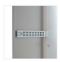
**Description:** The DIP profile system is a 40 mm wide and 25 mm high profile, which can be mounted on the enclosure depth. It can also be used in combination with CLPF and CLPK profiles. Two rows of holes patterns for cage nut fixing and self-tapping screws are provided. DIP profiles are not compatible with adjustment in depth of the mounting plate.
