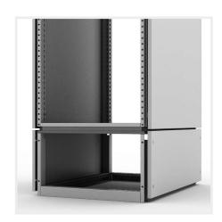
**Description:** For fixing and routing of cables or mounting of busbar. Identical hole pattern to the enclosure's frame makes all relevant accessories (e.g. CLPF, CLPK, etc) possible to mount. Fixed to the base of the enclosure by M12 screws (provided). Standard height 300 mm (200 mm available on request only).
