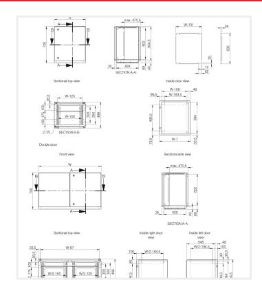
This stainless steel combinable console system, MPCS, has a IP 55/56 protection degree. It includes three interchangeable sections, top, desk and bottom. The system is very flexible and the various possible combinations can meet many design requirements. The ergonomic design of the top and desk units allows for easy installation and access to HMI-equipment, plus increases the mounting space available. This console can be installed in virtually any environment, grade dependent.
