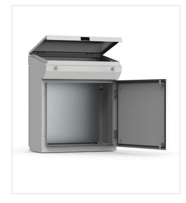
The mild steel compact console, MPG, in a IP 55/56 protection degree is available off the shelf. It has a hinged desk panel, and the ergonomic design allows for easy installation and access to HMI-equipment. It also increases the mounting space available. Stainless steel top panels may be used as an alternative when the console is exposed chemical agents, etc.
