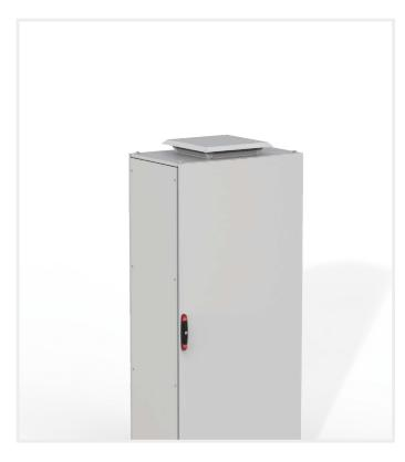
This roof filter fan, RFU, with either a IP 33 or 54 protection degree, to be mounted on the enclosure's roof, is easily mounted with a click-in feature. Thus, no surface needs to be used on the door. Component failure and downtime is eliminated as water and dust are prevented from entering the enclosure. The filter fan's reliable motor guarantees constant ventilation within each enclosure on which the fan is installed.
