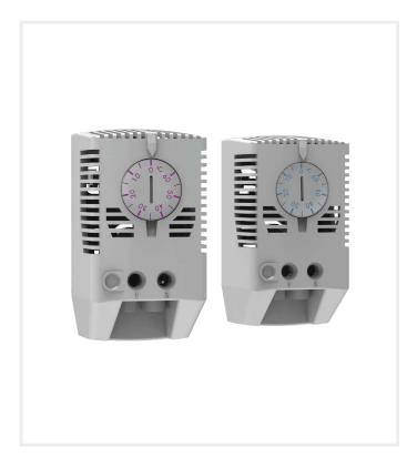
This adjustable temperature thermostat, ETR, for any enclosure, with either a normally open (NO) or normally closed (NC) contact, is used to control installed devices. Such devices could be a filter fan or a fan heater, that should turn on or off at the required temperature level, set by the user. The result is reduced operational cost.
