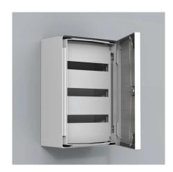
**Description:** Front cover plate with cut-outs for DIN components. Distance between UFCP and enclosure door: 39 mm; 49 mm for UCP750 and above. Reversible mounting position, to increase the distance between UFCP and enclosure door by 30 mm. The mounting frame with DIN rails UMFxxxx must be ordered separately.
