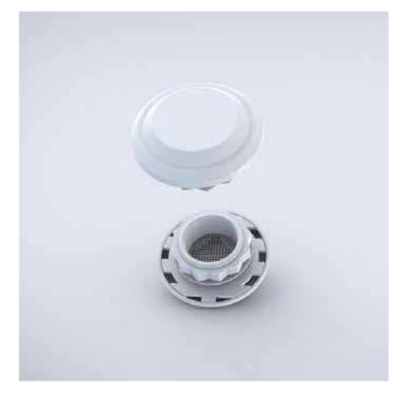
The pressure compensation plug equalises the pressure that occurs, due to temperature differences, inside the enclosure with the outside environment, while reducing the risk of dust entering the enclosure.
