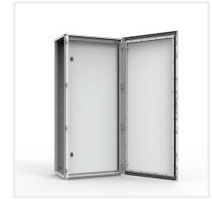
**Description:** Inner door provides a hinged mounting surface for equipment behind a standard or glazed front door. A mounting space of 80 mm, is available between the doors when the inner door is in the most forward position. Can be adjusted in depth by steps of 25 mm. The mounting plate remains usable behind the inner door. The door is equipped with two double-bit 3 mm locks.
