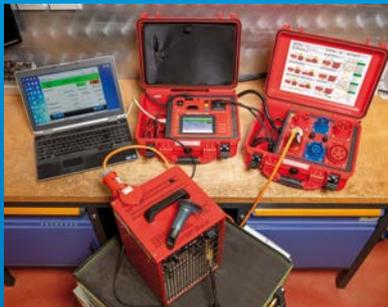
testing of a three-phase fan heater
