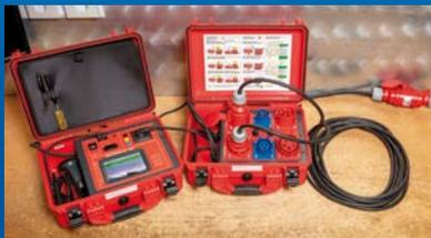
testing of a 5-pin CEE extension
