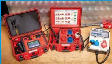
testing of a mobile power distribution with RCD
