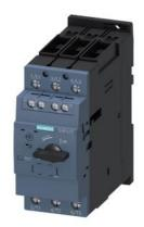
Circuit breaker size S2 for motor protection, CLASS 10 A-release 28...36 A N-release 520 A screw terminal Standard switching capacity with transverse auxiliary switches 1 NO+1 NC
