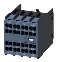
auxiliary switch, on the front, 2 NO + 2 NC, 53/54, 61/62, 71/72, 83/84, current path: 1 NO, 1 NC, 1 NO, spring-loaded terminal, physically coded, only with contactor relays 3RH2140 and 3RH2440 combinable (according to EN 50011)
