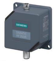
SIMATIC RF300; Reader RF350R (GEN2); RS422 interface (3964R); Without antenna IP65, -25 to +70 °C, 75x 75x 41 mm, can be operated with: ANT 1, 3, 3NO, 8, 12, 18, 30 special variant ATEX (Zone 3G/3D) and IECEx (Gc/Dc) for Zone 2/22.
